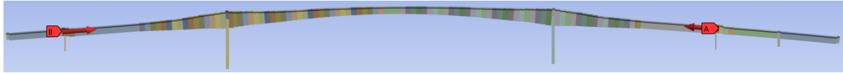
Figure 50: The post tensioning system simulated by two opposing remote forces on each end of the main span
