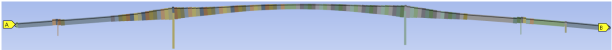
Figure 49: Remote supports on each end of the bridge, allowing no translation in x, y, z and no rotation about x, y. Allowing only rotation about z axis.
