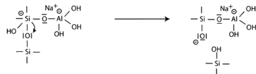
Figure 3: Formation of intermediate silanol ( \text{Si-OH} ) and basic siloxo ( \text{Si-O}^- ) [21]
