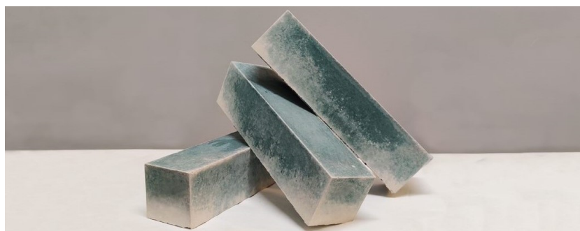
Figure 7.1: Greening effect on freshly demoulded DM8-REF samples
