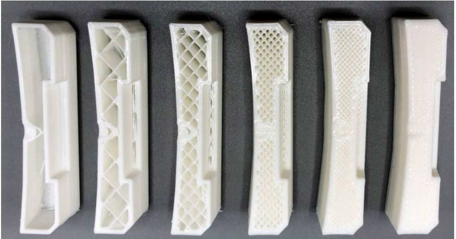
Figure 2: Cross-section of 3D printed parts with different infills [17]
