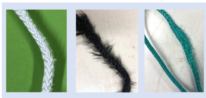
FIGURE 5: Nylon ROPE, PET STRAND AND PE ROPE, ALL AFTER WEAR.
