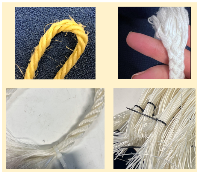
FIGURE 6: FROM UPPER LEFT: Sisal STRAND (WITH WEAR), Viscose ROPE, Bio-R ROPE AND Bio-D MONOFILAMENTS.
