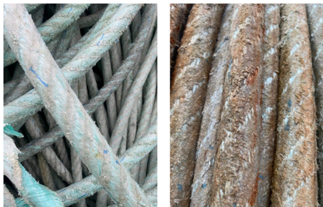
FIGURE 3: USED SEINE ROPES WITH VISIBLE WEAR.
