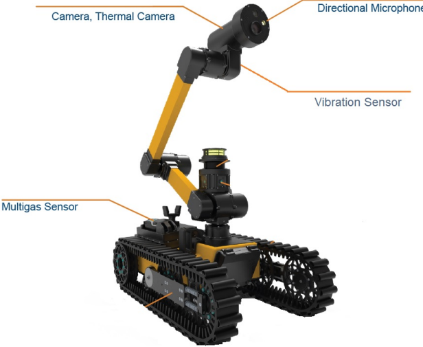
Figure 3.2 Illustration of sensors and instruments installation on a robot
