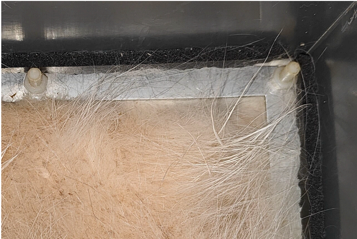
Figure 9. Photograph of an arctic fox pelt mounted in the conductivity measurement device. Pelt is clamped down and mounted onto the standard material by threading the eight holes made in the pelt using a scalpel blade, over eight plastic screws and attaching the aluminium frame tightly using bolts. A black insulative sealing strip can be seen along the edge of the frame.
