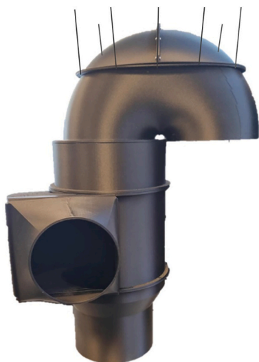
Fig. 11. The 3D printed SPRICE spray collector.
