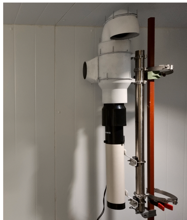
Fig. 12. SPRICE spray collector mounted on top of R. M. Young automatic precipitation gauge (model 50202).
