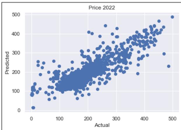
Figure 7 Scatter diagram showing the result of a combined time-space prediction model where input is a record set from 'SE3', 'DK1', 'Oslo', 'Bergen', 'NL', 'BE', 'AT', 'GB' at time t-24 (hours) and output is prediction in NO 2 at time t (hour).
