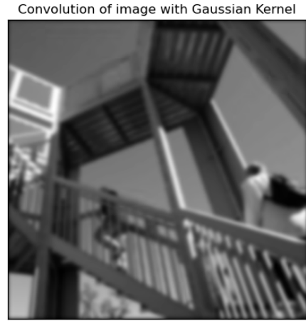
(b) Resulting image after performing convolution with a Gaussian Kernel, leading to smoothing or blurring of the original image.
