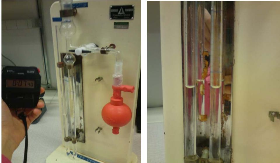
Figure 11. The Blaine apparatus
