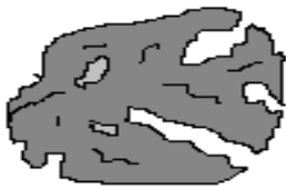
Figure 7. A cross section through a particle is made for an illustration of both open pores and closed pores. The closed pores inside particle does not reach surface as illustrated by light grey color. Open pores are seen reaching surface.
