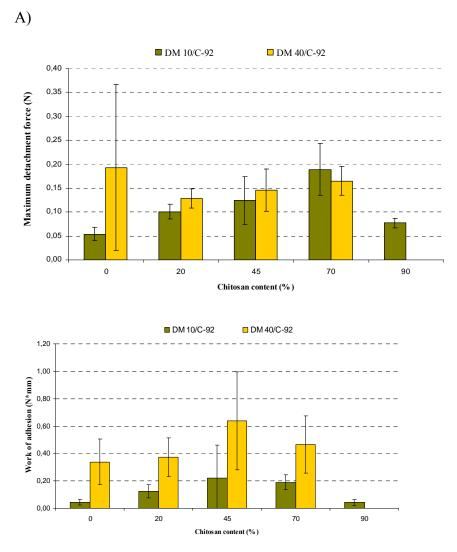
Figure 22: Mucoadhesion of 11 mm tablets to cow vaginal tissue for various combinations of chitosan:pectin ratio A): Maximum detachment force B) Work of adhesion. Data presented as mean  $\pm$  SD (n=3). (n=10)
