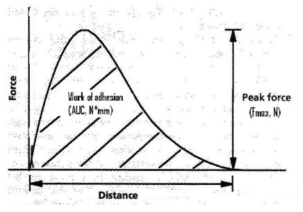
**Figure 13:** Modified illustration of force-distance curve defining work of adhesion and the peak force (Hagerstrom et al., 2004)
