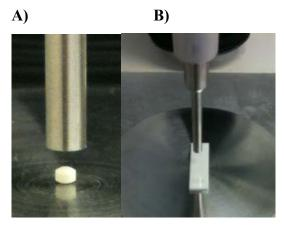
Figure 9: Illustration of A) measurement of height of a mini-tablet. B) Calibration for distance with calibration block.
