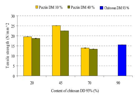
Figure 30: Tensile strength of various pectin type (DM 10% and 40%) and varying degree of C-92
