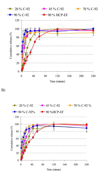
**Figure 24:** Dissolution profile of metronidazole (10% w/w) from different combinations of chitosan to pectin. Pectin grade used DM 10 %. Hydroxypropylecellulose added as reference A) VFS pH 4.5 B) VFS pH 6.8. Data presented as mean  $\pm$  SD (n=3).
