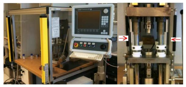
**Figure 5:** A) Schmidt ServoPress 450 A) Compression modul from IBR. Red arrows indicate the position of sensors which measures the distance
