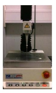
Figure 8: Illustration of crushing strength measurement of mini-tablets by using Texture Analyser.
