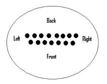
Figure 7: The filling of mini-tablet dies was done by placing the powder back, front, left and right.
