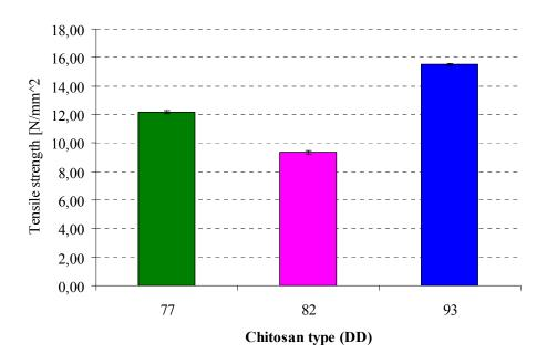
**Figure 28:** Tensiles strength based on height of 5 mini-tablets containing various chitosan types (DD 77%, 82% and 93%) Data presented as mean  $\pm$  SD (n=5).
