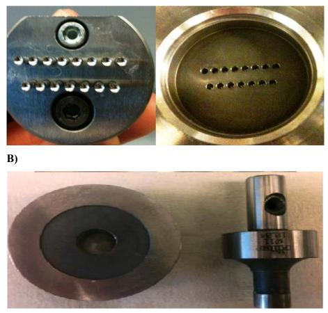
Figure 6: Tablet tooling A) 2 mm, concave multiple mini-tablet tooling. B) 11 mm flat-faced punch.
