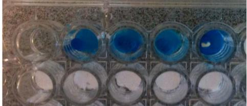
**Figure 15:** Photo of test set up: 96-titeplate with filter, sensient blue solution and mini-tablets. Fully coloured mini-tablets, confirming the end point of the test, can be seen in the back row,
