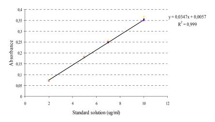
Figure 34: Standard solution of metronidazole in ammonium acetate buffer pH 4.5
