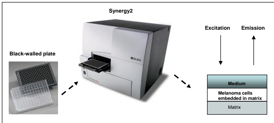
Figure 10. Schematic presentation of measurement of intensity of a DsRed signal. The DsRed labeled cells cultured in 3D (right) in black-well plates (left) were analyzed by a plate reader “Synergy2” (middle) measuring the DsRed fluorescence after excitation at 530nm.
