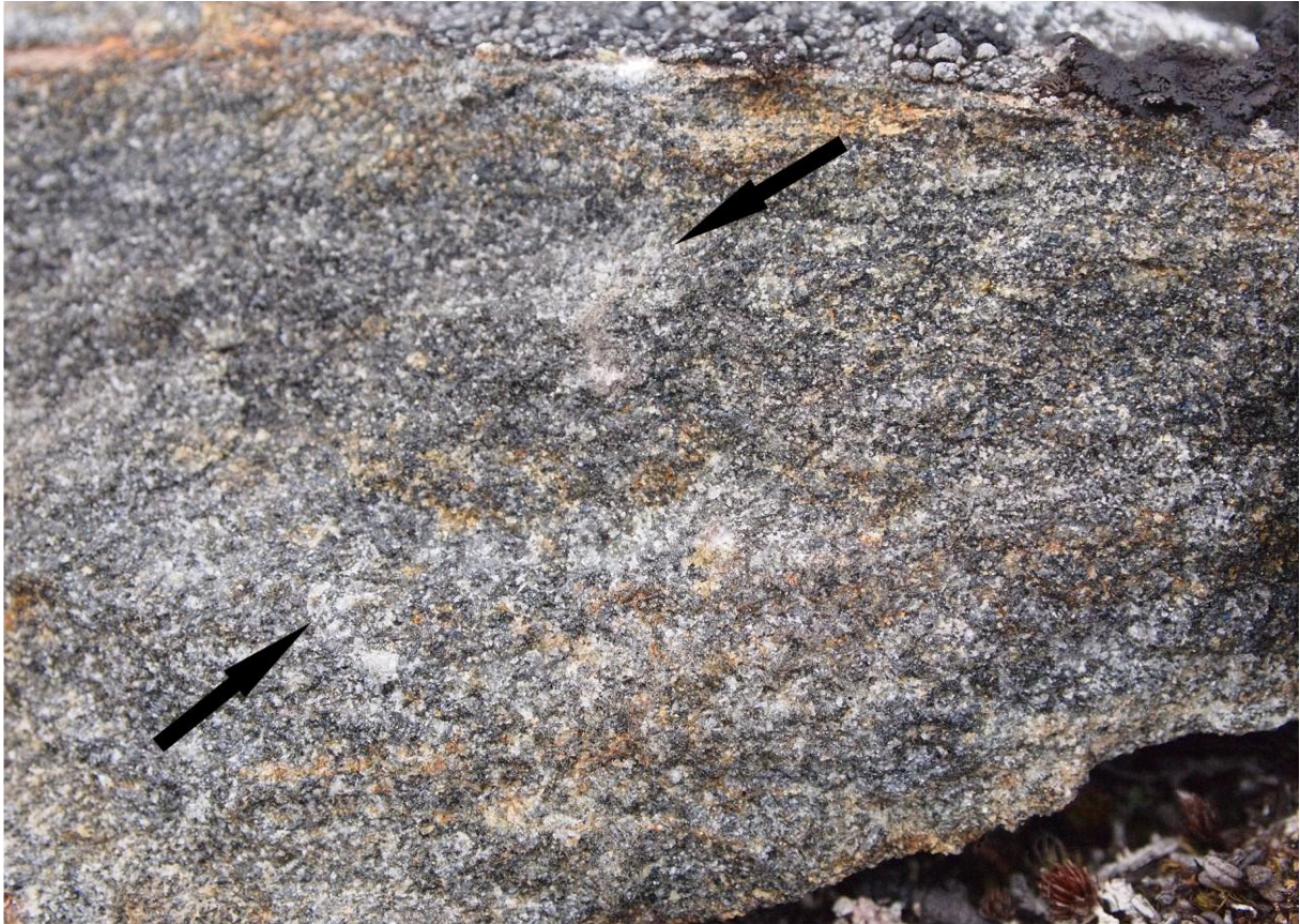
Figure 3.1-5: Image of the cpx-garnet amphibolite. Note the fine grain size and low coherence. Arrows mark examples of residual cpx which are light green in color. Base of image: ~10cm.
