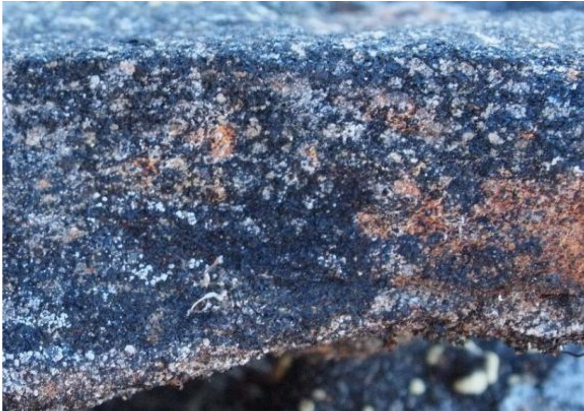
Figure 3.1-6: Close-up of the amphibolite of the Tromsø Nappe. Note the bluish tint of the fresh sample. Base of image: 5cm.
