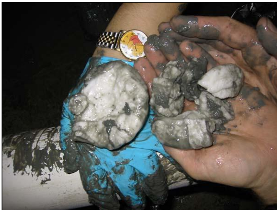
Figure 1-2: Chunks of gas hydrate recovered from the Gulf of Mexico in 2002 (from Winters and Lorenson, 2002).
