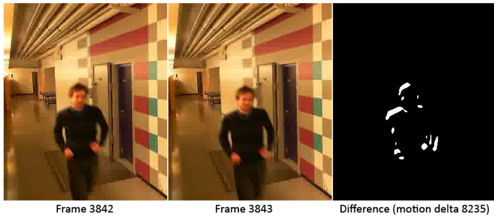
Figure 6.2: Two frames from the video stream and the difference between them. The absolute difference represented in this image is calculated to be 8235.
