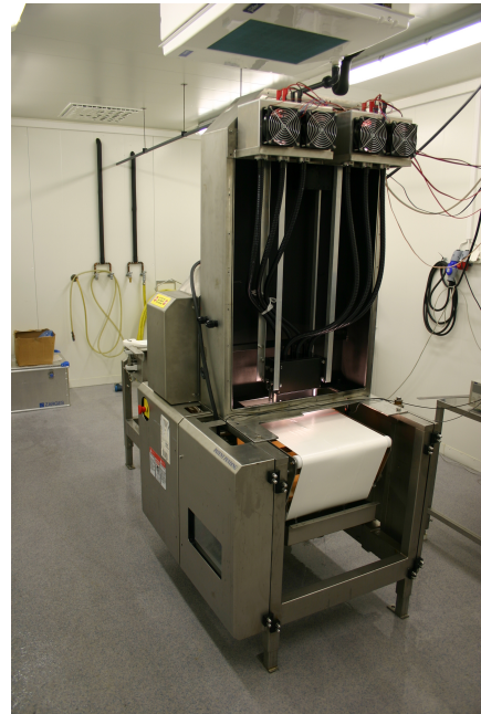
Figure 3.3: (a) A sketch showing the design and dimensions in mm, of the hyperspectral imaging setup for cod fillet inspection, and (b) a photo of the machine with the front cover removed. The light sources are connected to the two fiber lines through the black fiber cables seen in the photo.
