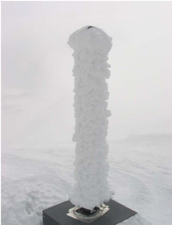
Figure 3.2: An ice load measuring stick. The ice is distributed around the whole rod keeping a somewhat cylindrical shape [Drage, 2005].
