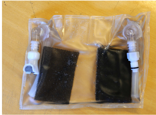
Figure 1.3: Water bolus used in this project. The black areas are open cell filter foam with two different thicknesses.
