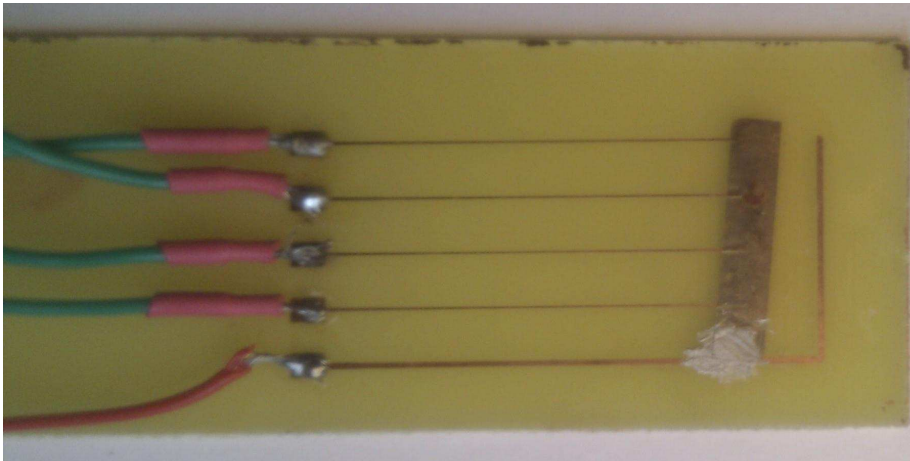
Figure 4.6: Circular transducer PCB. The golden strip to the right is the conductive top layer. On close inspection, the four transducer apertures are barely visible through it.
