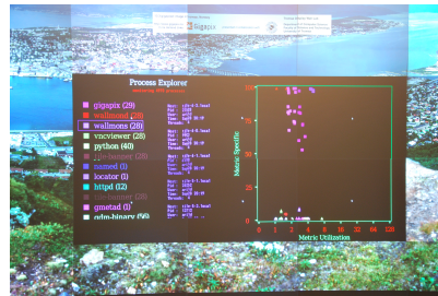
Figure 1: WallMon running on the Tromsø display wall. WallMon's visualization runs on 3x2 tiles, while an image of Tromsø is rendered in the background. Moving symbols within axes represent different performance metrics of processes running on the display wall cluster.
