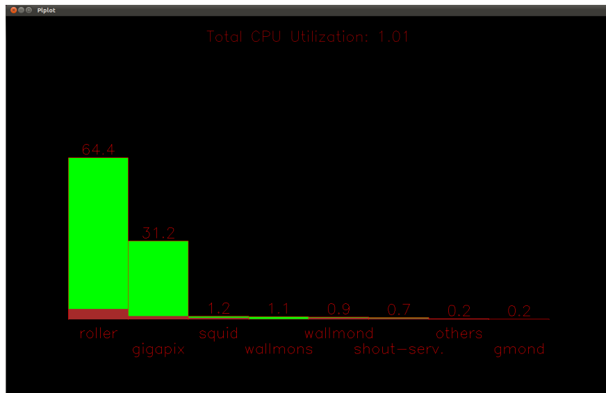
Figure 5.1: Early visualization prototype based on bar charts in WallMon. The chart shows the relative, aggregated user- (green part of bars) and kernel-level (red part of bars) CPU utilization of processes of equal name on the Tromsø display wall cluster, and aggregated CPU utilization of the entire cluster (located on top of the chart). The charts are sorted in descending order, with the process group with the most utilization to the left. Only 8 process groups are shown in the chart; the group others contains aggregated utilization for all other process groups.
