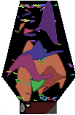
Figure 3.8: The LavaPS interface to process visualization. Each blob represents a process.
