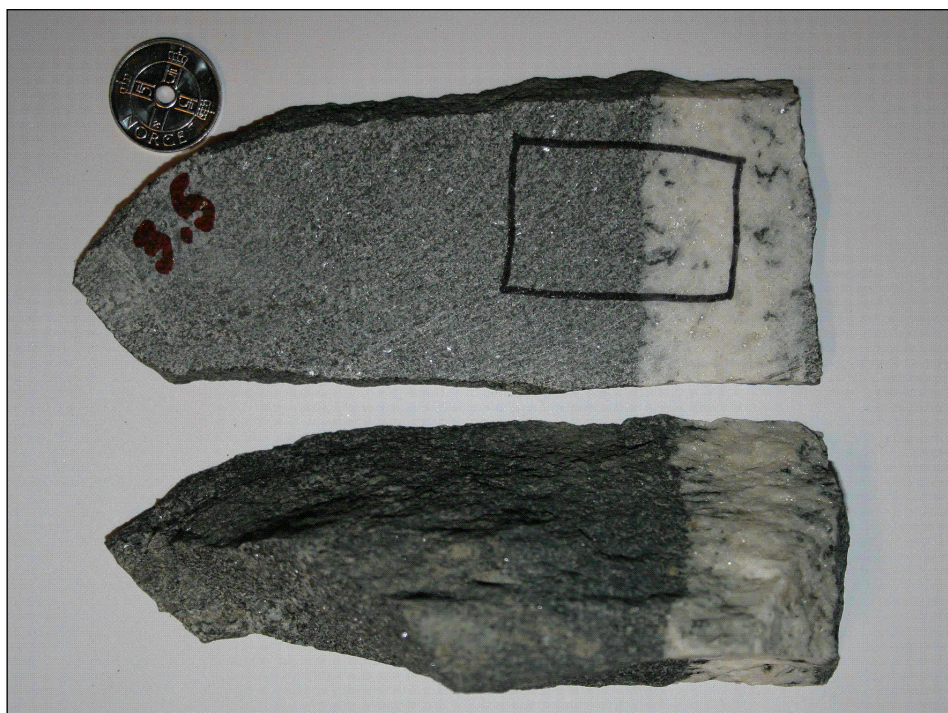
Figure 3.13: Image of sample 3.5 showing dolerite dyke with sharp contact towards felsic dyke. Foliation is weak and oblique to dyke edge. Black box is for thin section preparation. Diameter of coin = 2cm.
