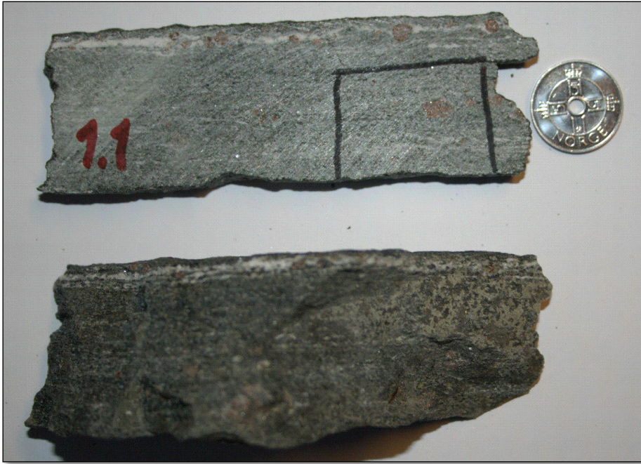
Figure 3.10: Sample 1.1 of foliated Cpx-Grt bearing amphibolite with porphyroblastic texture, and leucocratic vein. Black box is for thin section preparation. Diameter of coin= 2cm.
