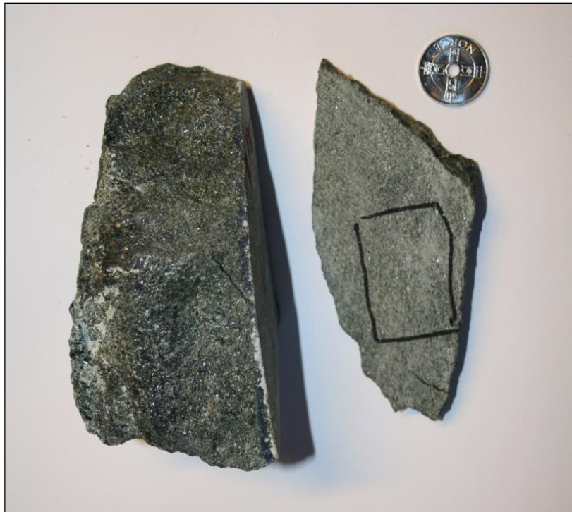
Figure 3.16: Image of sample 4.13 showing a weakly foliated variety of the amphibole-rich rock. Black box is for thin section preparation. Diameter of coin= 2cm.
