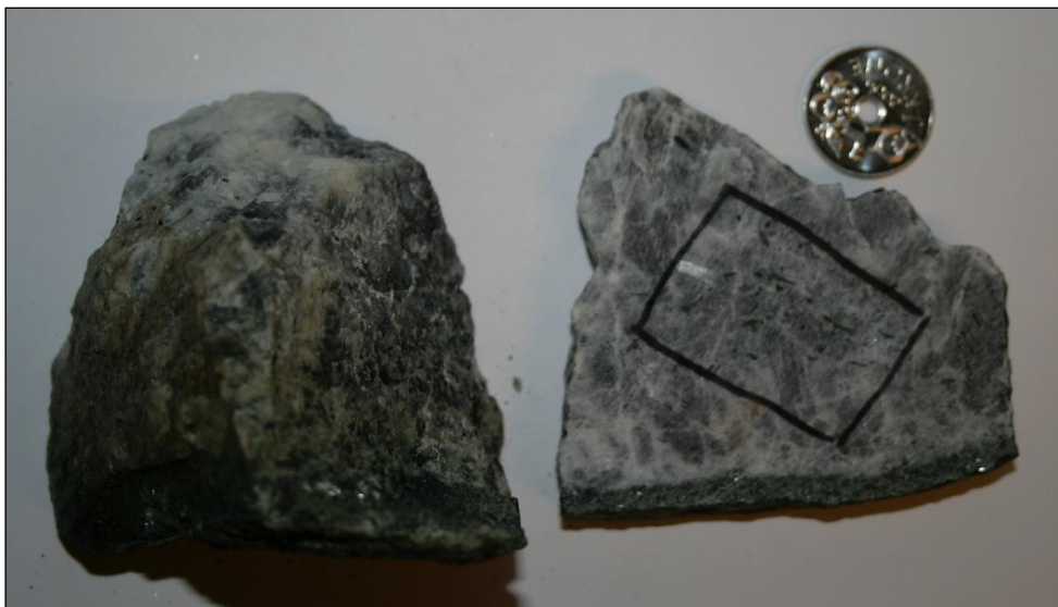
Figure 3.5: Sample 4.24 showing a coarse-grained, purple-grey variation of felsic dykes with white veinlets. Black box is for thin section preparation. Diameter of coin= 2cm.
