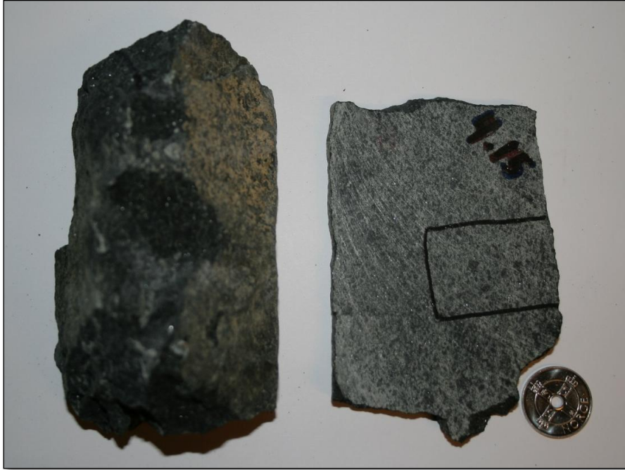
Figure 3.18: Sample 4.15 of massive serpentinite with brown weathered surface. Black box is for thin section preparation. Diameter of coin= 2 cm.
