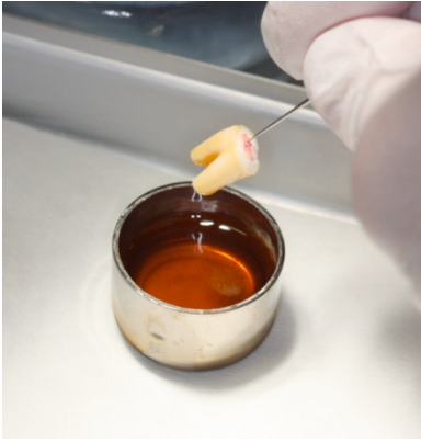
Fig. 1. The illustration shows how the specimens were covered in wax in preparation for dye immersion.
