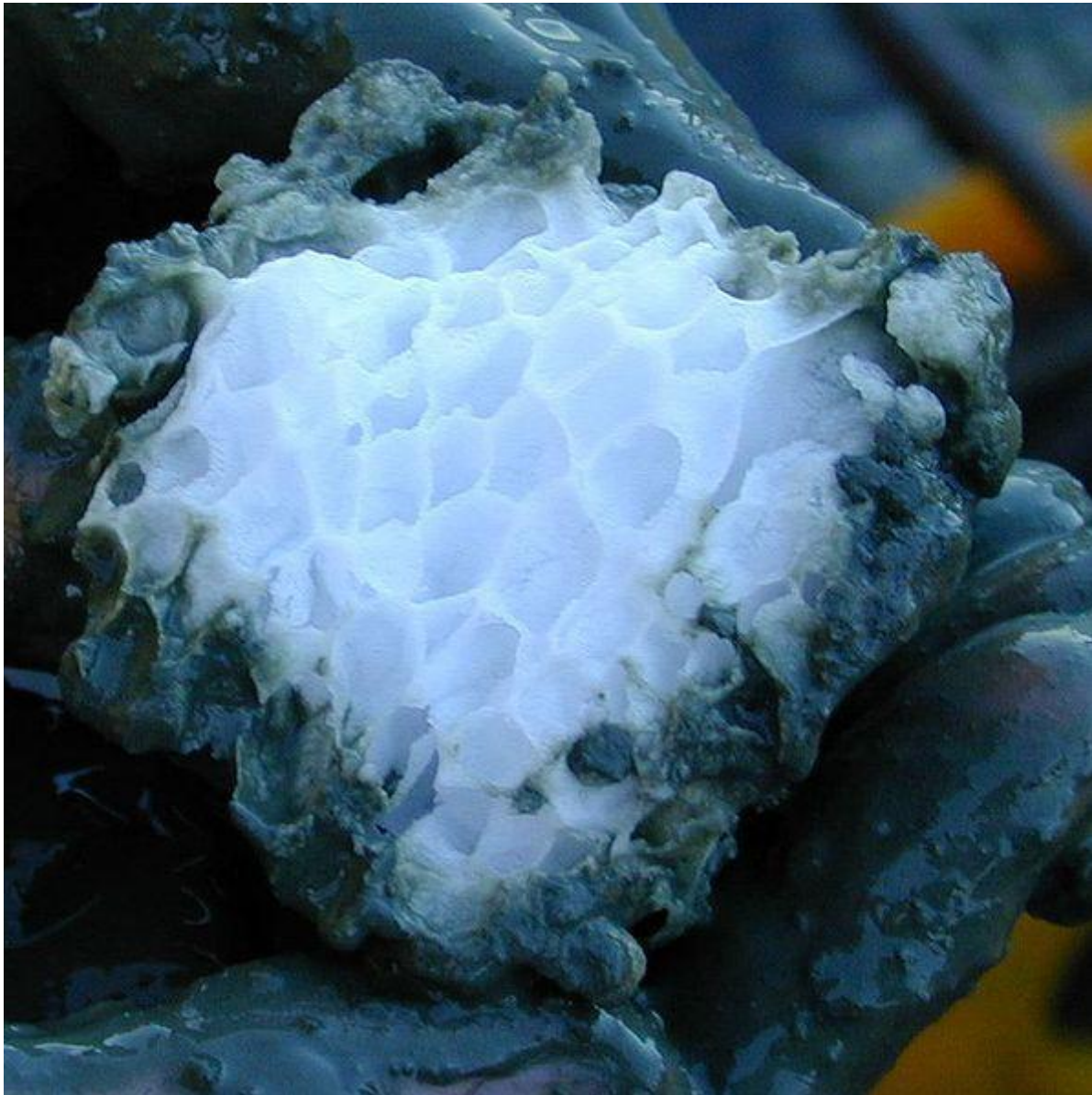
Figure 11. Gas hydrate recovered from an embedded hydrate structure of a sediment ridge offshore Oregon, USA. Gas Hydrates are not stable under atmospheric pressure and will release gas and water if not kept under high pressure and low temperature (picture from: http://feww.wordpress.com/category/east-siberian-arctic-shelf/ ).
