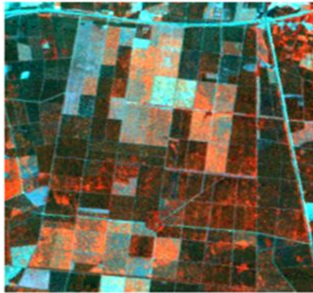
Figure 4.3: Color composite image of a portion of the Landsat data, band-4(Red), band-2(Green) and band-3(Blue).
