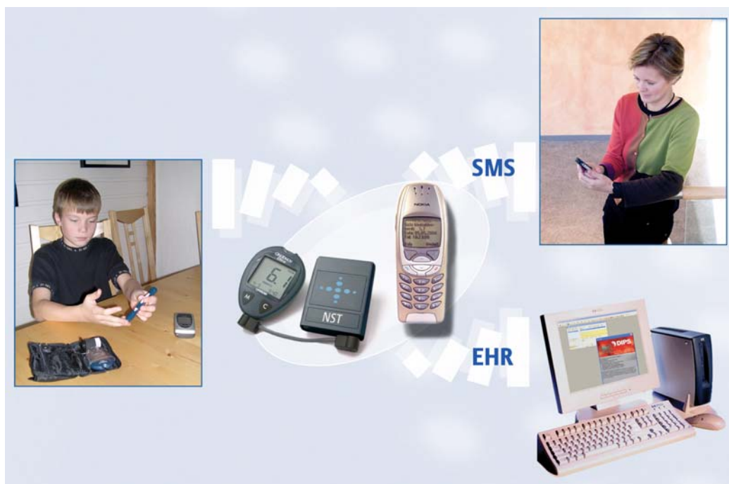
Figure 1: Automatic blood glucose data transfer to EHR and as an SMS to relatives. (Photo: Jarl-Stian Olsen/Hilde Pettersen NST)
