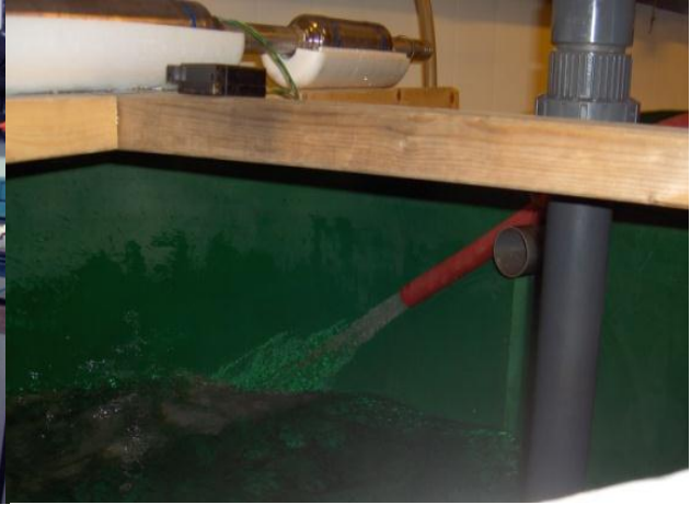
Figure 7 Filing tank at Dileka test setup at maximum flow of 20\text{m}^3\text{h}^{-1} .
