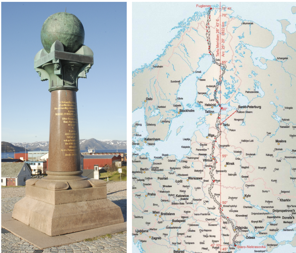
Figure 7. Left : the obelisk at Hammerfest is one of the geodetic points of measurement. The inscription reads 70° 40' 12" N, 23° 39' 48" E (photo CS). Right : Geodetic Arc map as displayed on site. Credit: National Land Survey of Finland.
