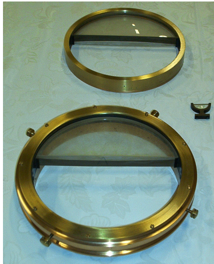
Figure 2. The lenses of Houzeau's heliometer. Photo C. Sterken.
