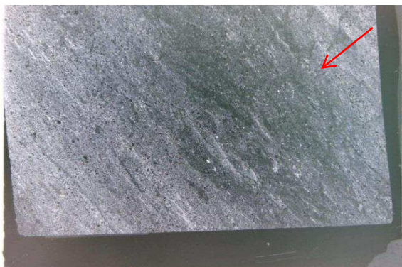
Figure. 3.1.22. Photo of NS-21 polished thin-section. A red arrow shows the direction of increasing grain size.
