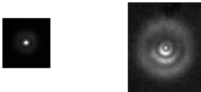
Figure 6.3: Particle with small and large ring. Both imaged 20 times. (Normalized images shown)
