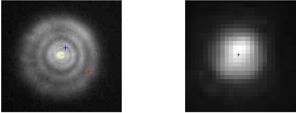
Figure 5.2: Left: Red and yellow show centre with regionprops for thresholds 50 and 70, respectively. Blue shows centre calculated with centerofmass, having subtracted 50 from the image. Right: Almost the same result for red, yellow and blue in this in-focus image.
