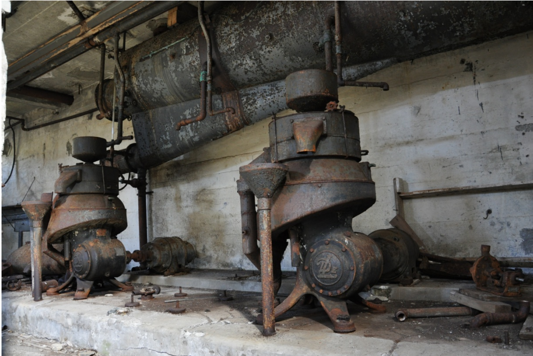
Figure 6: Oil centrifuges in the Ingólfur factory, Eyri (Photo: Þóra Pétursdóttir).
