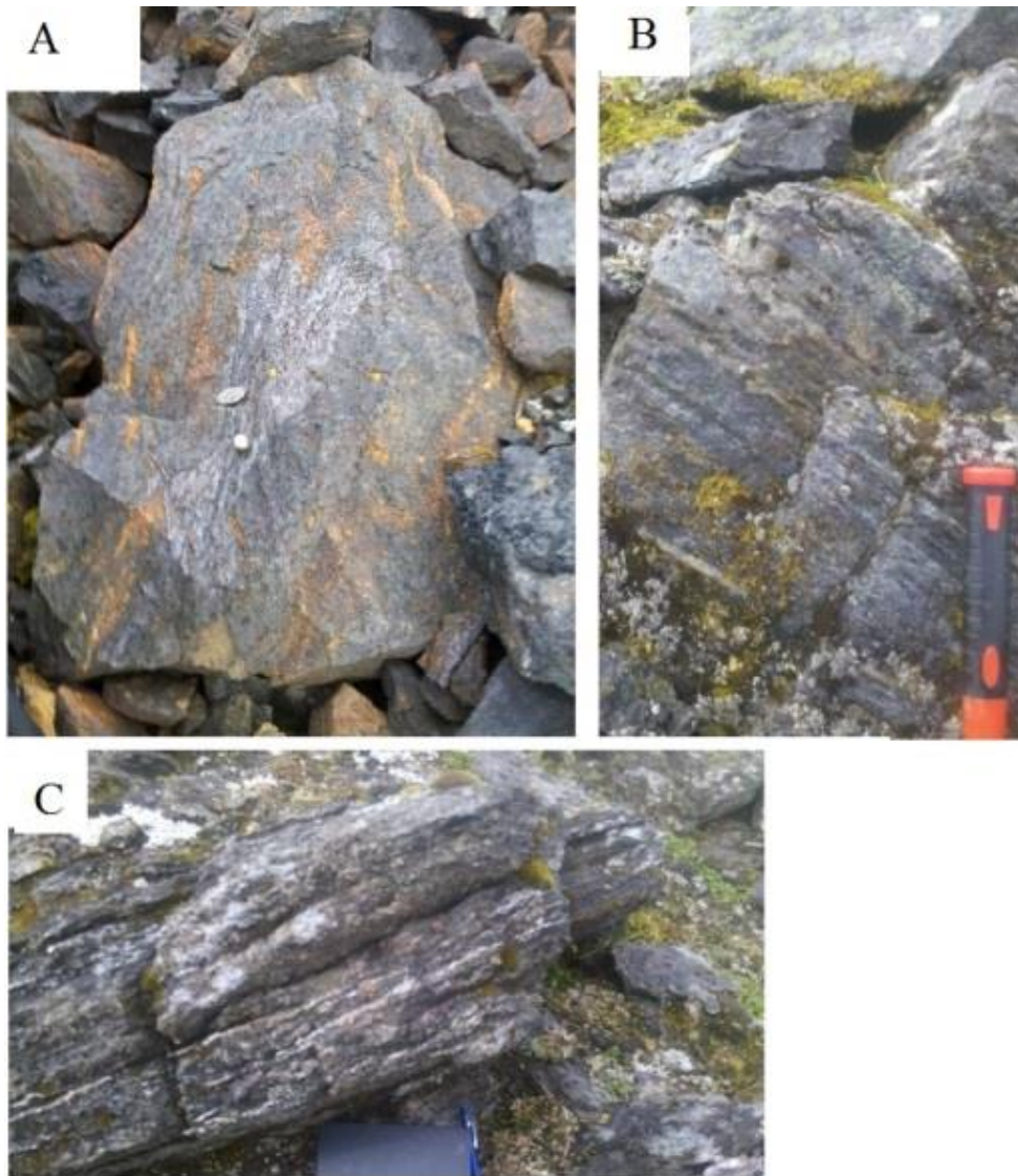
Figure 13 A) Close up of rock from the dump at the upper drift in Kalvebekli apparently made up of mostly magnetite and a yellow-brown weathering mineral. B) “Strongly” magnetic gneiss, magnetite, quartz and green (amphibole, pyroxene or epidote) bands, Solligangen. C) Amphibole Quartz Garnet Magnetite Gneiss, Solligangen.
