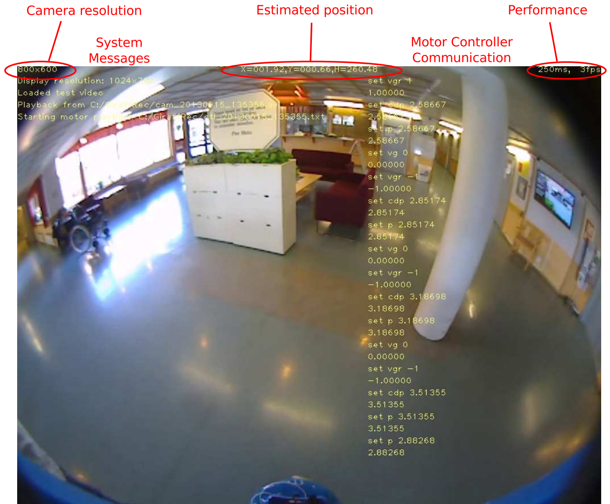
Figure 3.4.: Screenshot of a playback on a regular laptop, with UI elements marked
