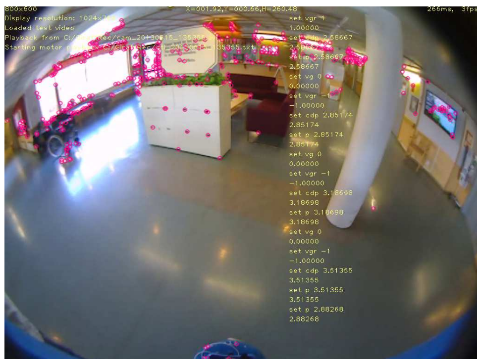
Figure 5.2.: Playback with FAST corner detector (corners highlighted with pink)
