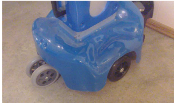
Figure 3.3.: Bottom of chassis. rear swivel caster, and right drive wheel.
