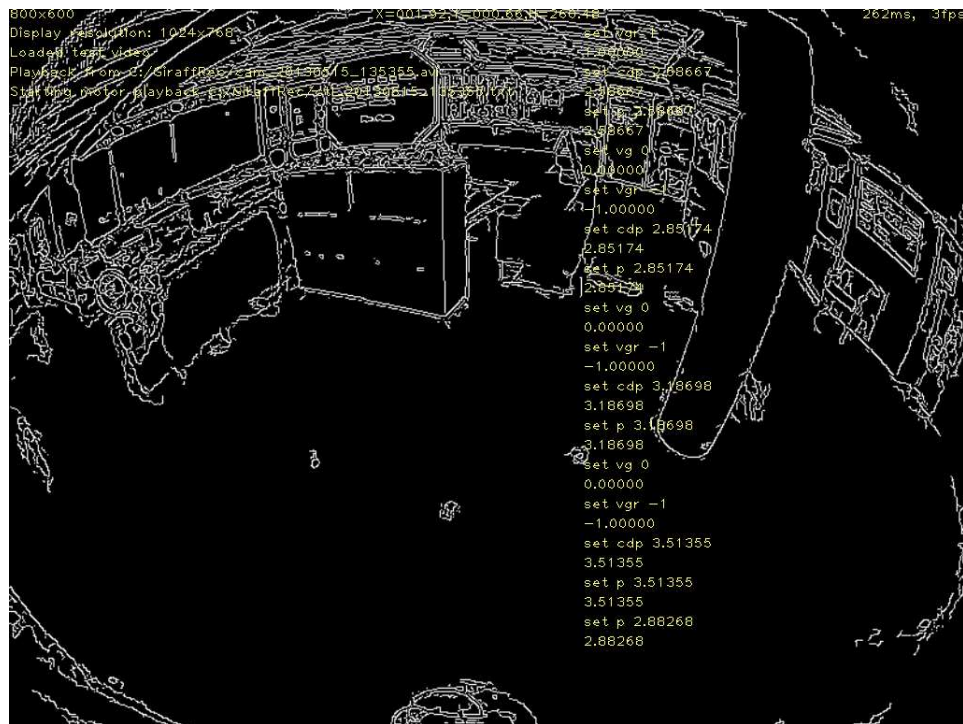
Figure 5.1.: Playback with Canny edge detector
