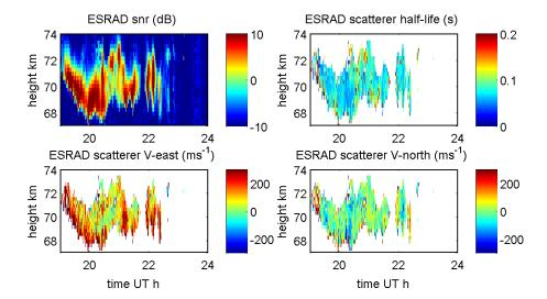
**Fig. 8.** Results of full correlation analysis of ESRAD data during the evening PMWE event. Top left panel shows signal-to-noise ratio, top right panel shows scatterer lifetime (time to decay to half power), bottom left panel shows eastward horizontal scatterer drift speed, bottom right panel shows northward horizontal scatterer drift speed (all 300-m height resolution, 22 s average data, one profile each 64 s).
