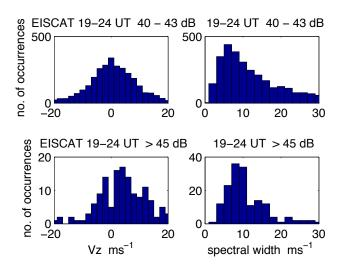
**Fig. 7.** Histograms showing the distribution of Doppler shifts and spectral widths for the EISCAT observations included in Fig. 5. The power interval 40–43 dB is chosen to represent echoes from the background ionospheric plasma, while power >45 dB is representative of PMWE.
