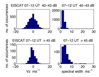
**Fig. 4.** Histograms showing the distribution of Doppler shifts and spectral widths for the EISCAT observations included in Fig. 2. The power interval 40–43 dB is chosen to represent echoes from the background ionospheric plasma, while power >45 dB is representative of PMWE.
