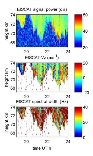
**Fig. 5.** EISCAT observations covering the strong PMWE event in the evening sector. Upper panel shows radar echo strength, middle panel shows echo Doppler shift (positive towards the radar), lower panel shows echo spectral width (all 30 s integrated data).
