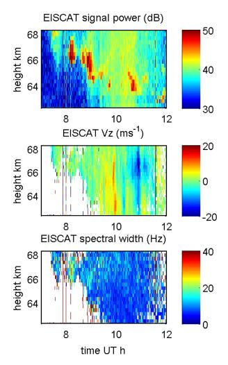
**Fig. 2.** EISCAT observations covering the strong PMWE event in the pre-noon sector. Upper panel shows radar echo strength, middle panel shows echo Doppler shift (positive towards the radar), lower panel shows echo spectral width (all 30 s integrated data).
