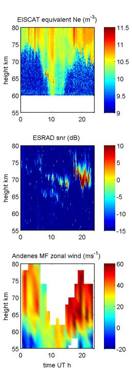
**Fig. 1.** Overview of observations on 10 November 2004. Upper panel shows equivalent electron densities measured by the EISCAT 224-MHz VHF radar (1-min integrated data), middle panel shows radar echo signal to noise ratio measured by the ESRAD 52-MHz radar (600-m height resolution, 25 s average data, one profile each 64 s), lower panel shows zonal winds derived from measurements by the Andenes 2-MHz radar (time resolution 1 h, height resolution 4 km, interpolation used for plotting).
