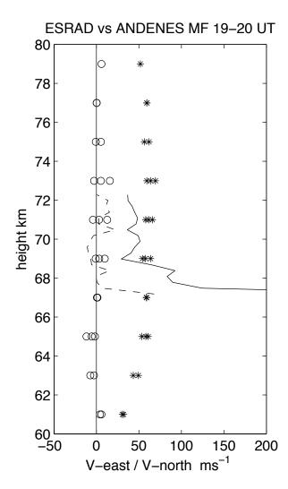
**Fig. 10.** Profiles of the results of ESRAD scatterer drift-speed analysis averaged between 19:00–20:00 UT (solid line is eastward drift, dashed line is northward drift), compared with winds from the Andenes MF radar for the same time interval (\* show eastward wind, o show northward wind). Both 30-min and 60-min average profiles are plotted for the MF radar.
