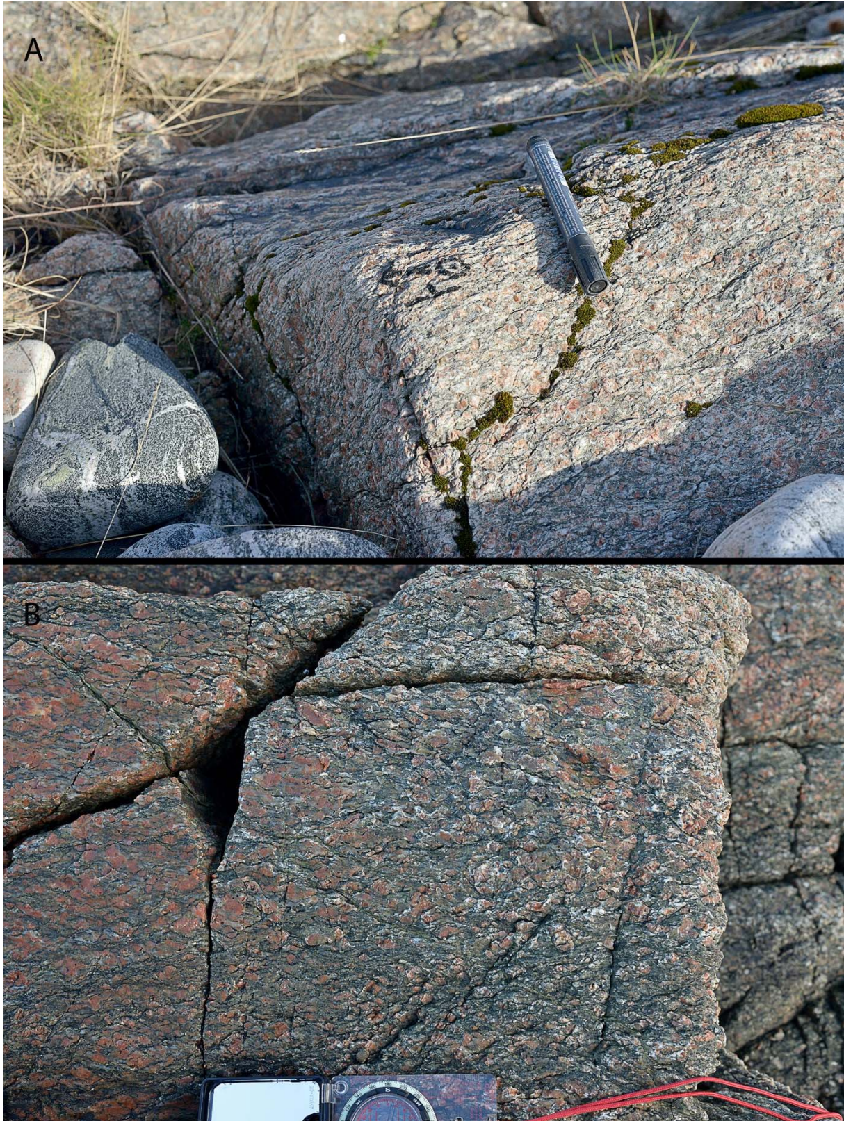
Figure 2-2: A digital photograph of the host rock. (A) Field appearance of the mostly unaltered rock, the picture is taken a few meters from a shear zone. Red 5-15 mm K-fsp phenocrysts are seen, where white areas are plagioclase and quartz. The foliation bands contains abundant epidote, quartz and chlorite and accessory minerals. Marker=14 cm. (B) A close-up viewing near perpendicular to foliation near a shear zone. The bands are thicker and contains more alteration products. Compass plate=10 cm.
