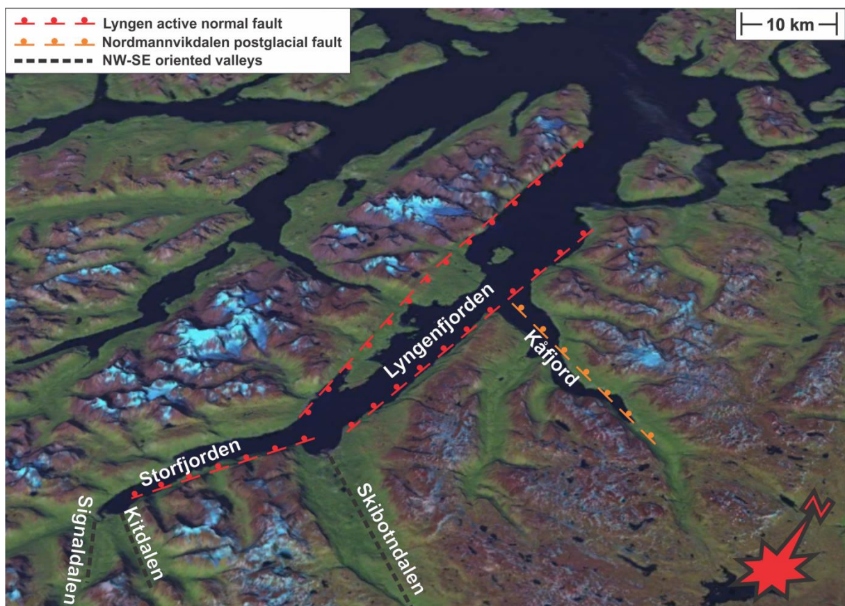
Figure 2.3: Map displaying both post-Caledonian and postglacial elements found adjacent to the study area. The red stippled line represents the NNE-SSW oriented Lyngen active normal faults. The orange stippled line gives the position of the NW-SE striking Nordmannvikdalen postglacial fault. The dots on the stippled lines indicate the dip of the faults. The black stippled lines show the location of some of the NW-SE oriented, structurally controlled, valleys in the region.
