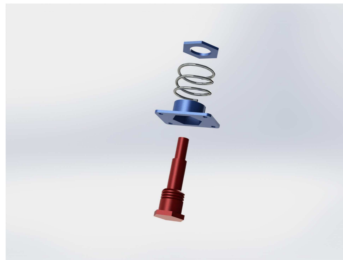
Exploded view of Damper
