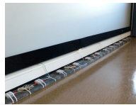
Figure 10. Cameras along the floor detect objects along the wall.
