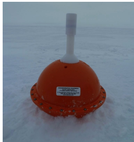
(d) Iridium Surface Velocity Profiler (ISVP) buoy. Image courtesy of S. Gerland, Norwegian Polar Institute.
