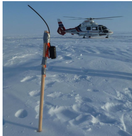
(c) GPS tracker mounted on a wooden stick. Image courtesy of S. Gerland, Norwegian Polar Institute.
