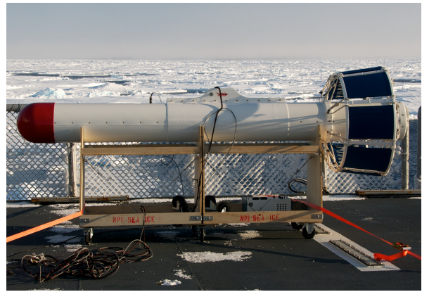
(b) Close-up of EM-bird. Image courtesy of A. H. H. Renner, Norwegian Polar Institute.
