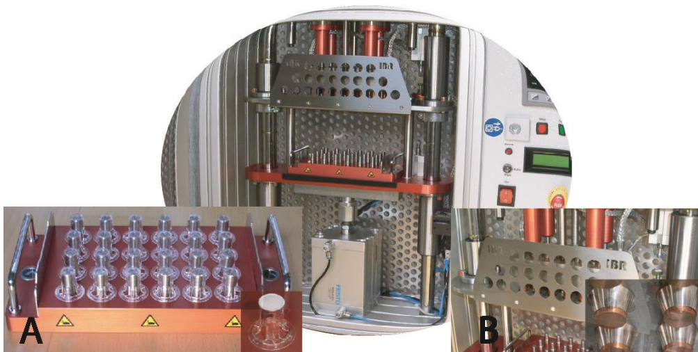
Figure 4.5: Pictures of the sealing machine IBR Heat-Press HP80-3500. A and B gives a closer look at the sealing part of the instrument.
