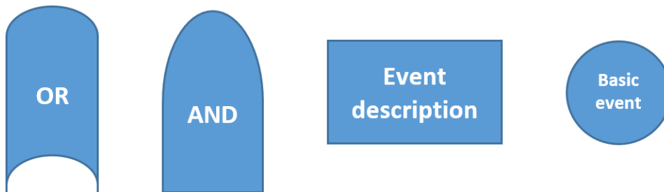
Figure 4.2: The most common gates and symbols used for FTA analysis; OR-gate, AND-gate, box for description of event and basic event.
