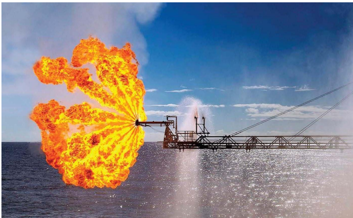
Figure 13; Evergreen burner (SLB, 2014)
