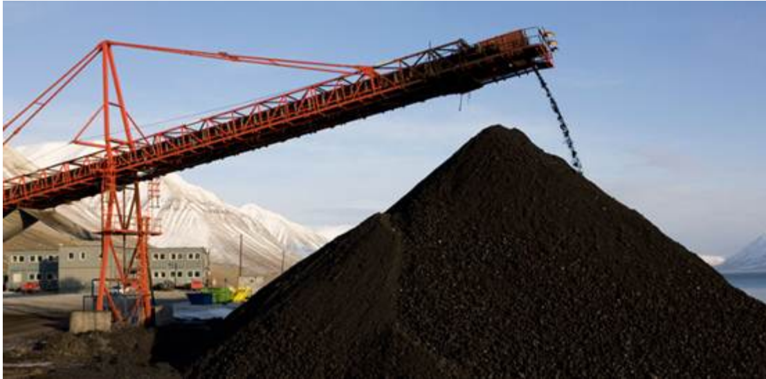
Figure 17 – The Stacker for the Svea coal mine
