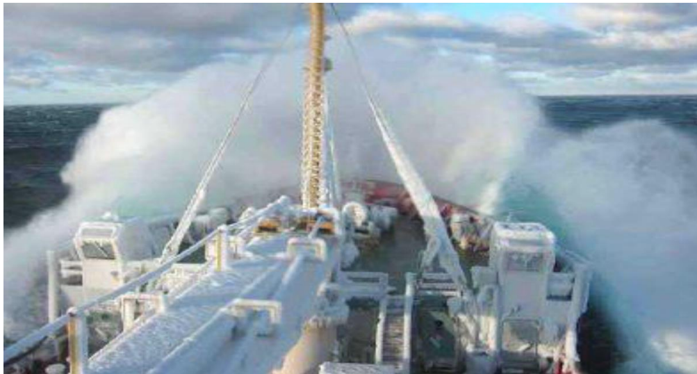
Figure 3.12 Sea sprays icing from waves and swells (Source: Canadian Coast Guard)
