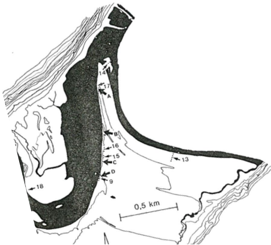
Fig. 4-9. Map of Sandbukta Beach, showing the four locations (A, B, C, and D) where erosion was measured from 1984-1985. From Fjalstad, 1986.
