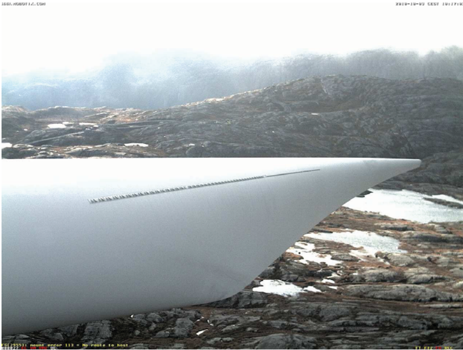
Figure 3.8: Clean blade imaged by web camera to illustrate contrast with the iced blade.
