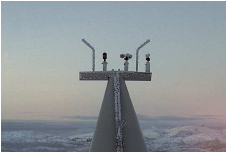
Figure 5.27: Rime ice visible on the sensors following the icing event Dec. 5.
