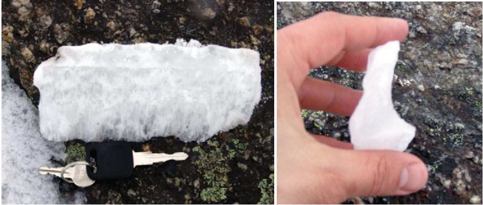
Figure 2.7: Glaze icing from a wind turbine blade.
