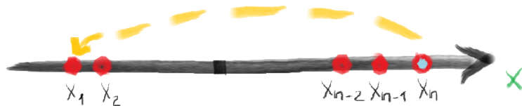
Figure 18: Applying Periodic boundaries on the plane: to calculate the value of a function at the point x_n (for the fourth order accuracy) we use two points from the left x_{n-2} and x_{n-1} , but then to make the right boundary periodic ‘a ring has to be closed’, thus we use the two first points x_1 and x_2 .
