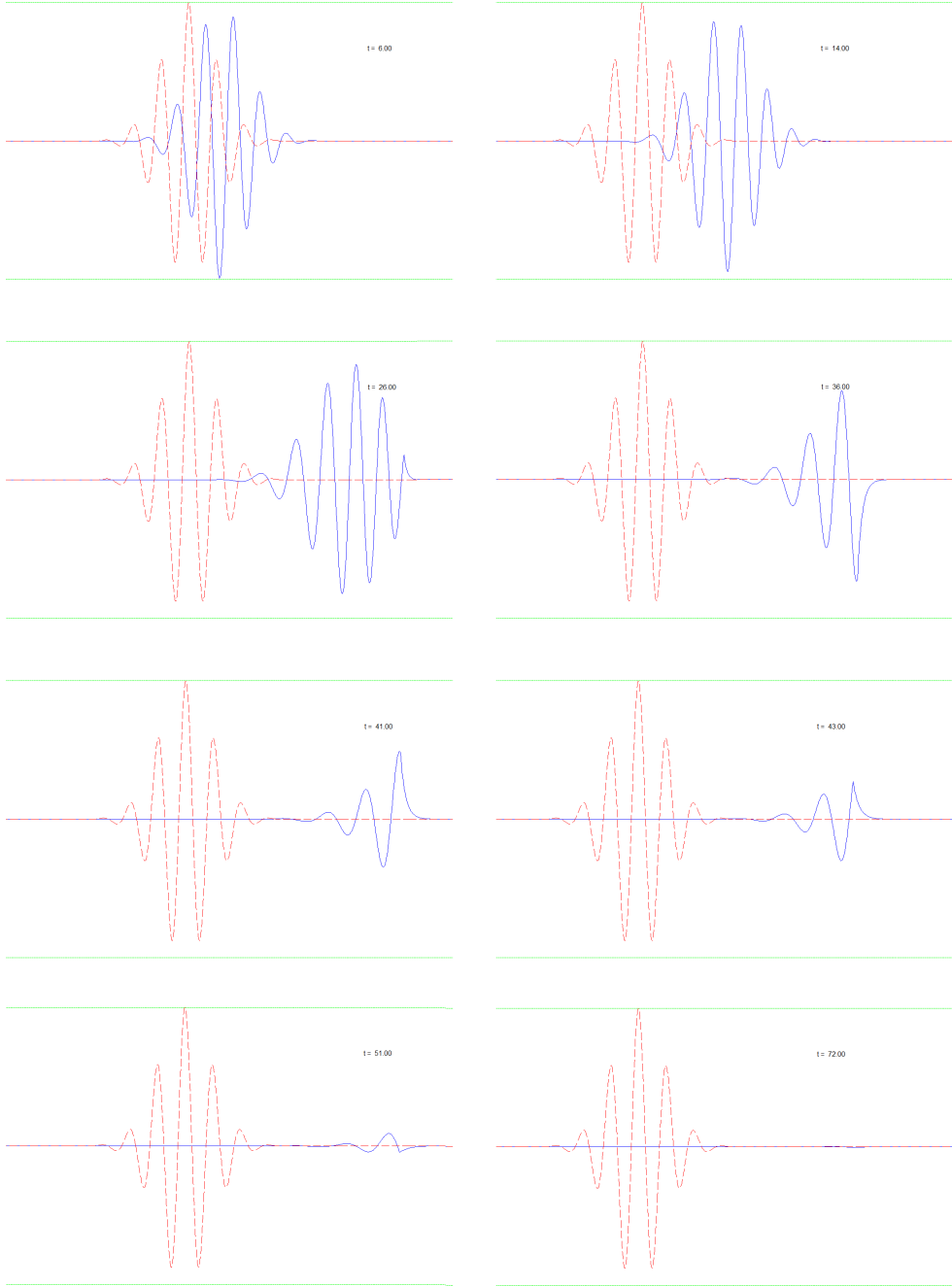
Figure 16: A wave packet (blue solid line) formed by \varphi_0 = e^{-\gamma(x-x_0)^P} e^{ikx} , with \gamma = 2 , x_0 = 0 , P = 2 , k = 12 , and boundary conditions: \varphi_{j=1} = \varphi(-L, t) , \varphi_{j=n} = \varphi(L, t) – set to zero. We can see (reading from left to right and then down) how a wave packet moves to the right ( k = 12 ), in accordance with a reduced Schrödinger equation (34) applied. Later, when it reaches PML of a form (Fig. 15), that starts at the point a = 4 , it gets absorbed. The red dashed line represents the exact initial function \varphi_0 (we used it to check the numerical solution). It is quite hard to notice any reflection on this scale, but on a bigger one, or when reducing the number of steps in calculations, we can observe small reflection. Though, we assume it to be negligible. The numerical approach used (code [A]) is based on Taylor's Expansion for the spatial derivative and a built-in ODE-solver for the time derivative of (34).
