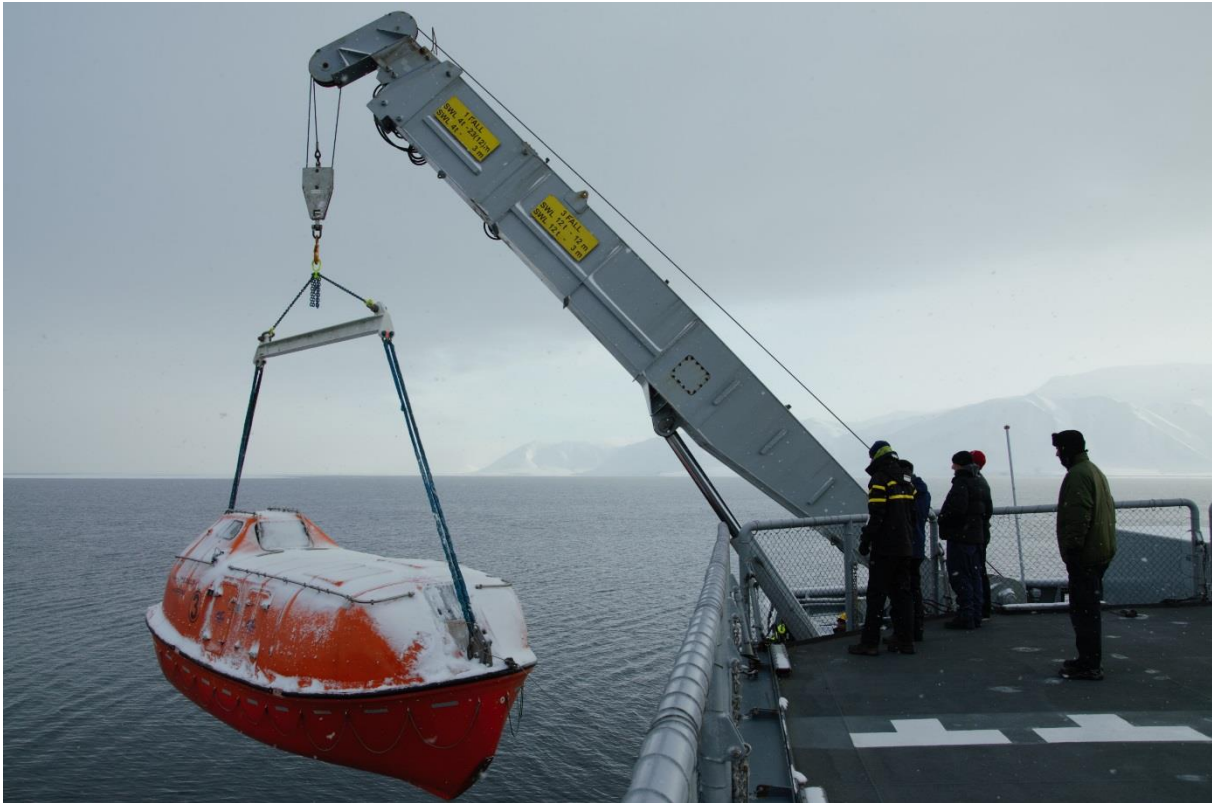
Figure 40: Lifeboat being lowered into the water with the deck crane. Photo © Jan Erik Jensen
