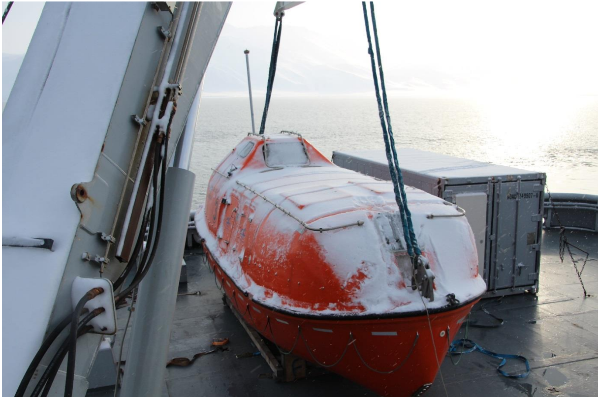
Figure 53: The lifeboat experienced snow accumulation during the test. Photo © Trond Spande
