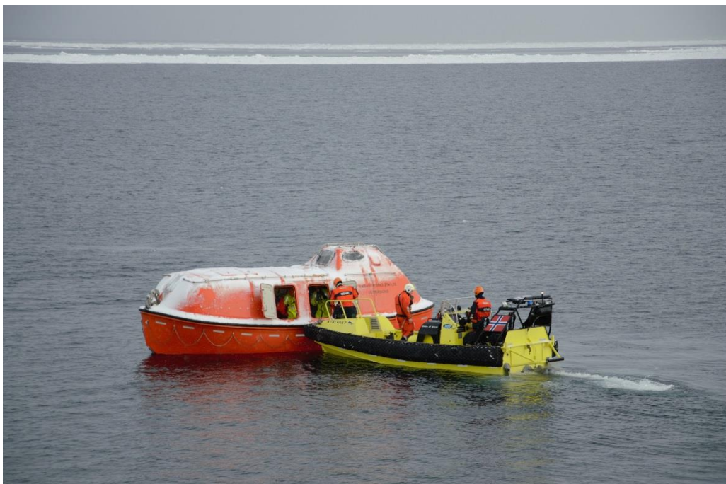
Figure 56: Lifeboat together with the MOB boat used as rescue vessel in the test. Photo © Jan Erik Jensen
