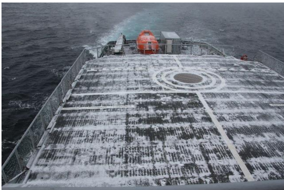
Figure 50: Snow accumulation on deck of KV Svalbard. Photo © Trond Spande
