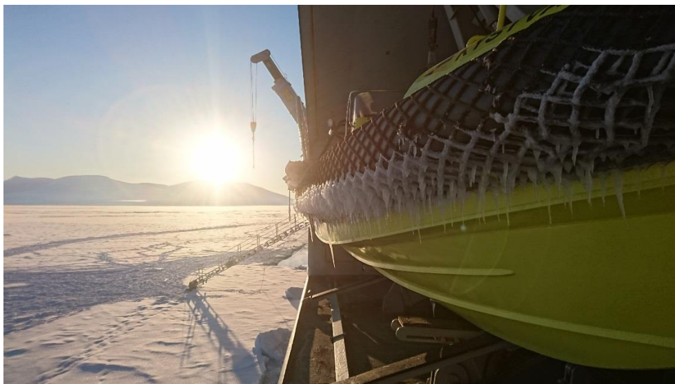
Figure 55: Icing on the MOB boat used during the test. Photo © Tord Nese
