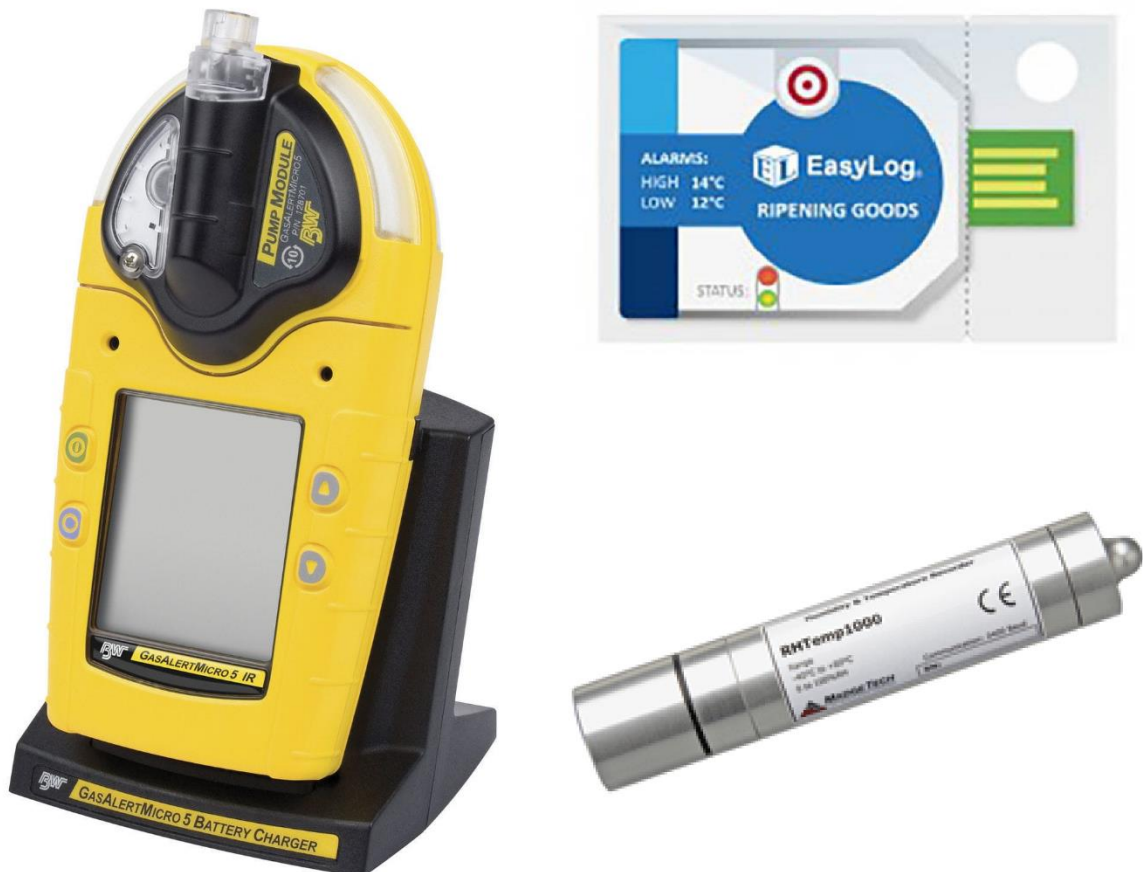
Figure 30: Logging equipment used during lifeboat test. Left: GasAlertMicro 5 IR gas detector. Top right: EasyLog EL-CC-1-003 temperature logger. Bottom right: RHTemp1000 humidity & temperature data logger
