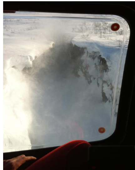
Figure 4.2-2 - Downwash in snow from a Eurocopter EC 135 machine. Photo: Håkon B. Abrahamsen
