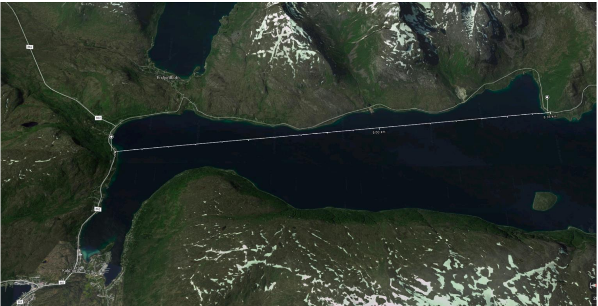
Figure 4.3-1 - Measurement of communication link for TRCs hexacopter (total distance 8.36km), created using google maps
