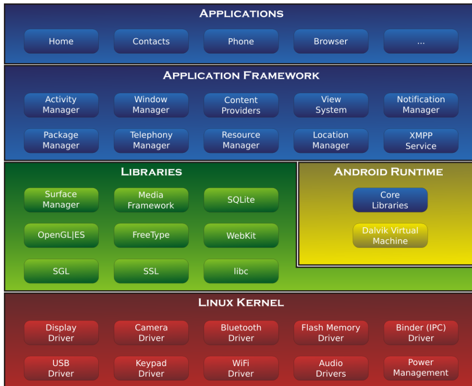
Figure 2.3: Overview of the Android system architecture [64].
