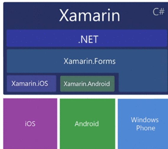
Figure 2.8: The Xamarin platform binds native iOS and Android SDKs to the .NET platform [79].
