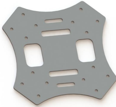
Figure 4.12 Power distributing board 2 solid modelling
