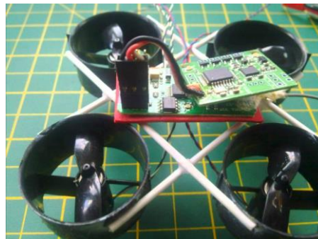
Figure 4.4 Custom made duct (Google image search on custom made ducts)
