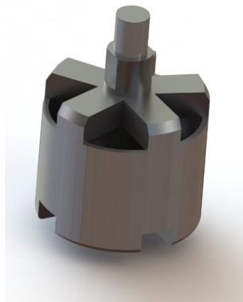
Figure 4.8 Motor model for quadrotor
