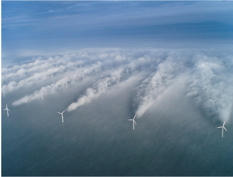
Figure 2.3: Illustration of wake effects in leeward side of wind turbines. The figure is borrowed from the National Oceanic and Atmospheric Administration (NOAA) [31]
